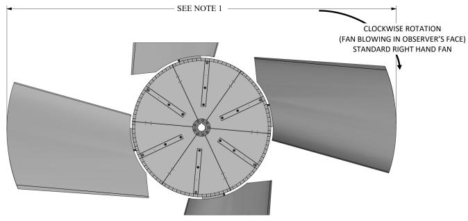
NOTE 1: MAXIMUM FAN DIAMETER EQUALS NOMINAL FAN DIAMETER. ADJUSTMENT OF  $\pm 1.5$  INCHES POSSIBLE AT INSTALLATION
