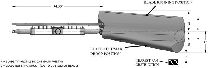
C = MAXIMUM DROOP POSITION OF BLADES AT 30° (C/L TO BOTTOM OF BLADE)
